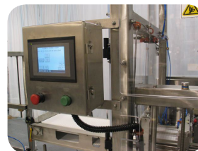
Stainless NEMA 4X HMI Enclosure with IP65 HMI
