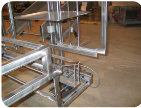
Angle and tube design - Zero tube penetration, no blind holes. Continuous weld, welded studs and sleeves used on frames.
