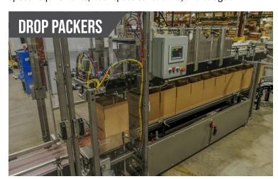
Engineered for both speed and accuracy, our drop packers are the pinnacle of high-throughput packaging. Products are presented above an open case before being gently "dropped". Our Drop Packers are available with an integrated case erector to minimize cost and footprint with models capable of speeds up to 30 cases per minute. We also offer standalone drop packers that can be fed from an independent case erector capable of speeds up to 50 cases per minute.
