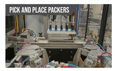
For more delicate or precise placement requirements, our Pick and Place systems offer unmatched performance. Utilizing an automated arm equipped with custom tooling, this system picks products from an infeed conveyor and carefully places them into awaiting cases staged on a parallel conveyor.
