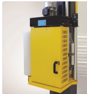
LP - Powered pre-stretch 240% (150%-200% - kit available as option)
