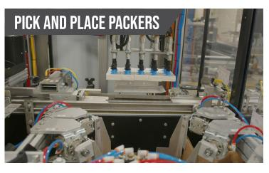
For more delicate or precise placement requirements, our Pick and Place systems offer unmatched performance. Utilizing an automated arm equipped with custom tooling, this system picks products from an infeed conveyor and carefully places them into awaiting cases staged on a parallel conveyor.
