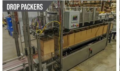
Engineered for both speed and accuracy, our drop packers are the pinnacle of high-throughput packaging. Products are presented above an open case before being gently "dropped". Our Drop Packers are available with an integrated case erector to minimize cost and footprint with models capable of speeds up to 30 cases per minute. We also offer standalone drop packers that can be fed from an independent case erector capable of speeds up to 50 cases per minute.
